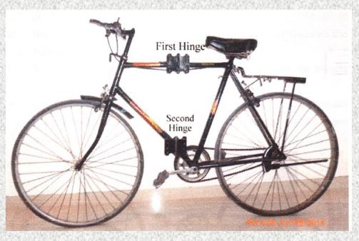
Conventional bicycles occupy sufficient space and hence providing one at work place or at home are quite difficult. They are probable to be exposed to the weather outside and do require frequent maintenance. With all such issues in the conventional bicycles, the next possible solution is the usage of foldable bicycle
