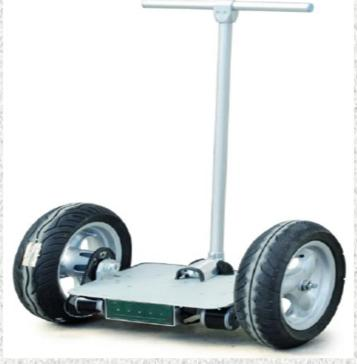
The Self balancing scooter is based on the principle of Segway Human Transporter where the velocity is controlled by the tilt of the driver. When the driver leans forward and backward, the scooter is running forward and backward. It is an intelligent vehicle which uses gyroscopic sensors detects the motion of rider, so that rider can accelerate, steer or brake the vehicle.
